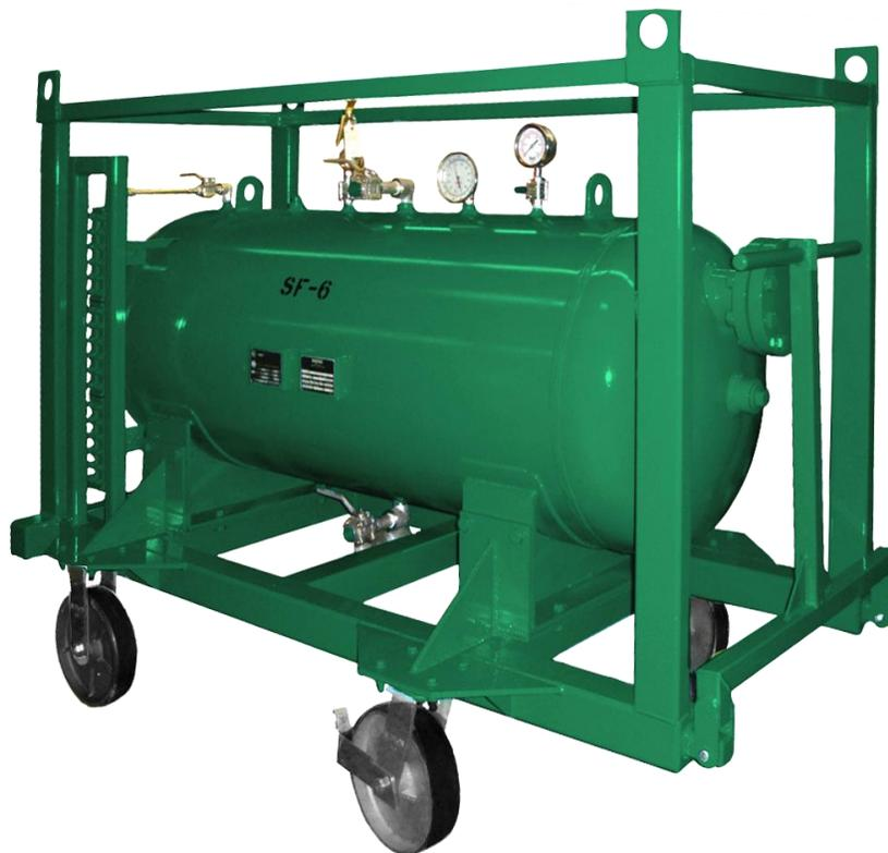
Various sizes of liquid SF6 storage tanks are available. Enervac's stationary or mobile Gas Storage Tanks are designed, fabricated and registered to the ASME code. Standard features include: Liquid level gauge, ASME relief valve, pressure gauge, temperature gauge, tank inspection flange, inlet and outlet valves. Mobile tanks are mounted on 12" (30 cm) casters with a tow bar.
