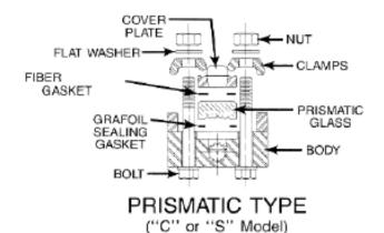
Note: 1) Prism side of glass must face inside of gage, as shown
