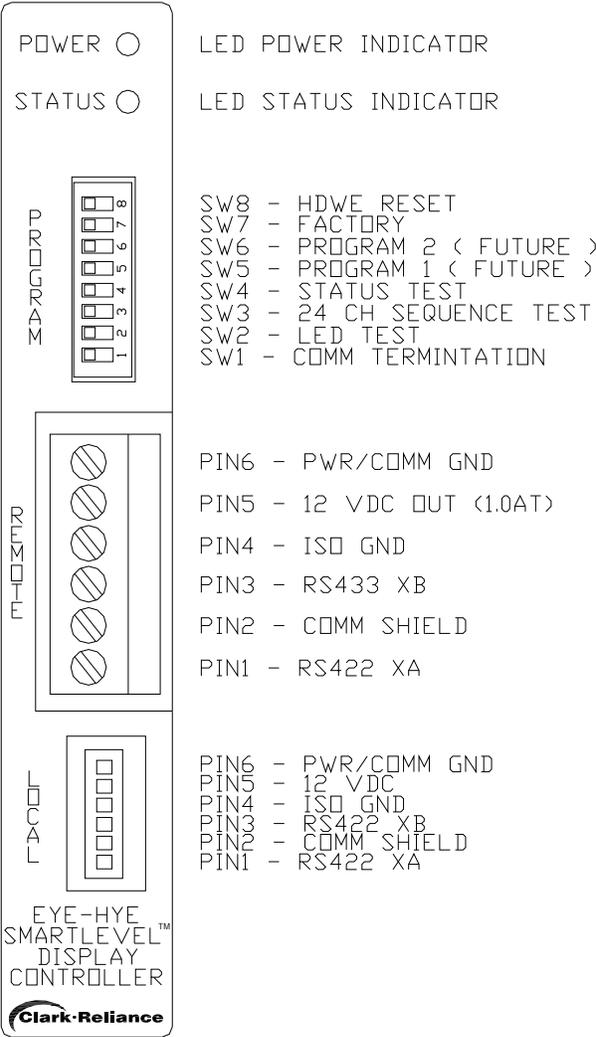
Figure 9 – LED Display Controller
