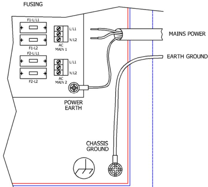
Figure 7 – AC Mains and Protect Earth Grounds
