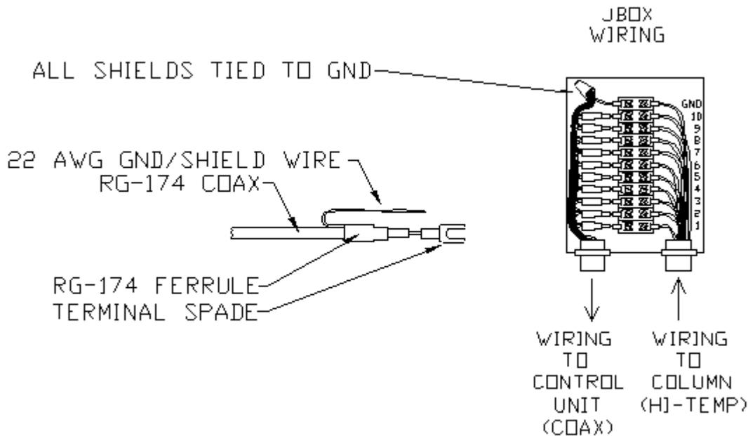
Figure 3 – Junction Box Wiring
