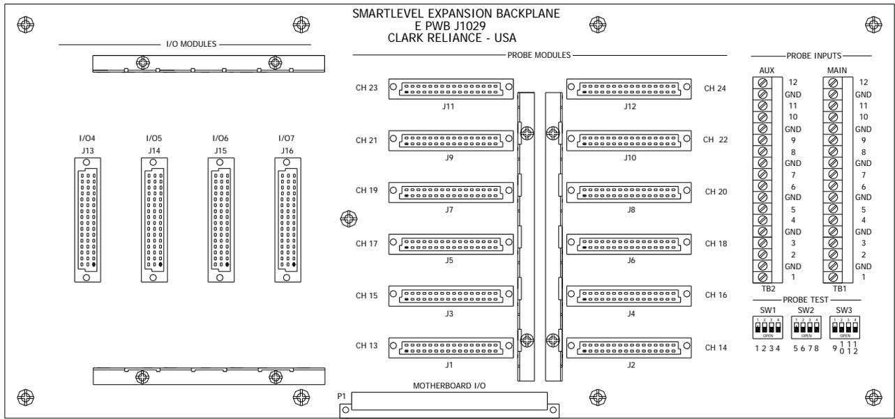
**Figure 23 – 24 Channel Expansion PCB**
