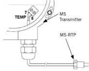
16 ft of cable provided. When the JMS-RTP is connected, the integral temperature probe is automatically overridden.
