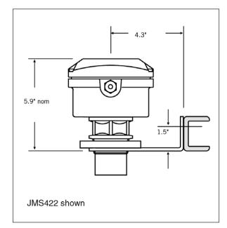
Note: Transmitters are not suitable for mounting in 2" NB pipe. A minimum of 3" NB is required. Use a plastic flange if mounting onto a tank or standpipe.
