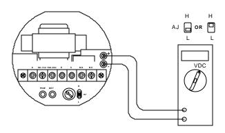
After adjustment, set the switch to H or L and make sure 8 - 10V DC can be read.
