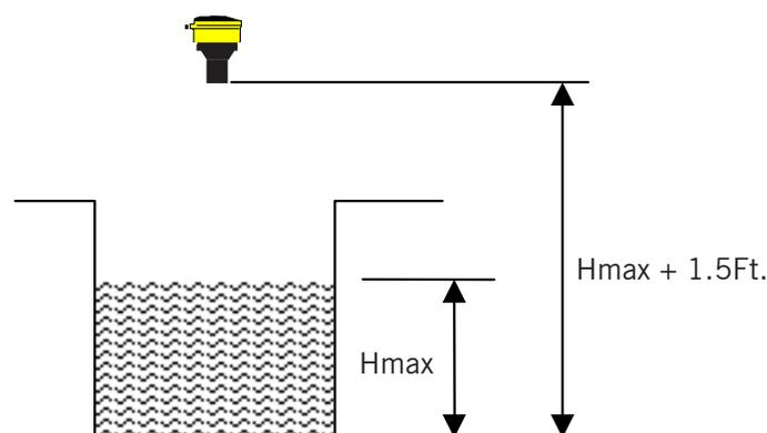
It is important to note that the bottom reference of the transmitter should be related to the centre of the invert of the primary device, NOT the distance to the channel bottom directly below the transmitter.
