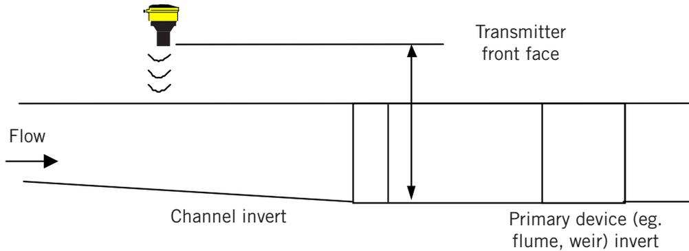
In addition to the above, when setting the bottom reference on a 'V' notch weir it is important that the true invert of the weir is taken and not the meniscus liquid level, which may be 3 to 4mm (1/8") above the true invert.
