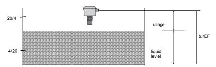
Before changing any of the default values, use blue button to scroll along to the next piece of information, which is the distance to target as measured by the MS422 from the front (transmit) face. This value is shown alternately with the text "diSt" to remind the user the MS422 display is in distance mode. You can now quickly check correct operation against a manual measurement if required.
