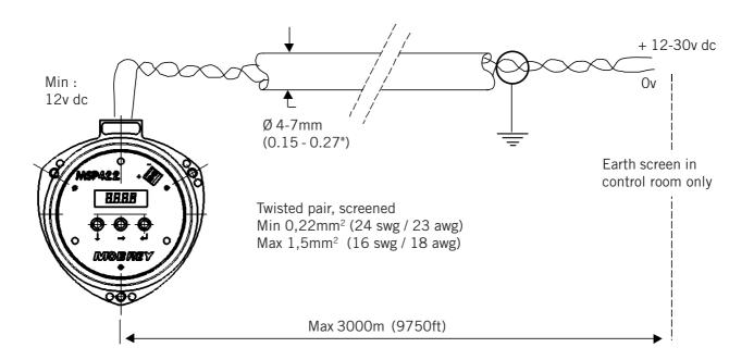
Multicore cable may be used, but it is recommended that each pair used to connect to an MS422 should be individually shielded.
