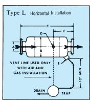
Separators have forged steel flanges, welded steel bodies and stainless steel element blades.
