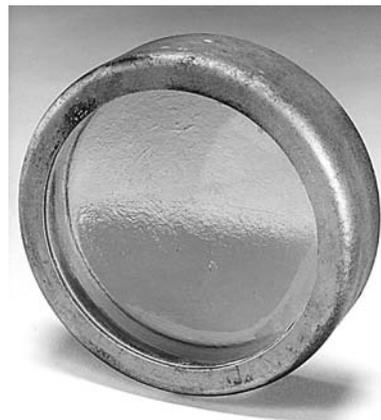
Borosilicate glass under attack by caustic
