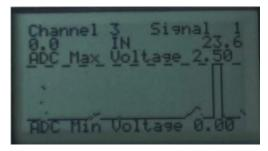
The graphs will show 23.6 inches of the graph of the sensor, measured in distance from the instrument head. When opening a graph, it is possible to change the starting point of the graph.
