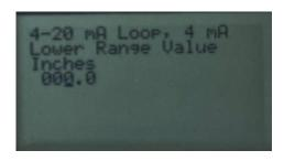
4-20 mA Loop, 20 mA Upper Range Value Inches 072.0 Enter the value desired for 4mA reading. Note this should be measured from the dead band set at the factory and marked on the sensor. Typically, the **Zero** is 000.0 for measuring the full (default) span.
