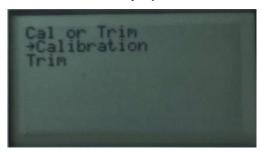
Two forms of One Point Calibration are available. **Calibration** is an emergency procedure to be used only if moving the instrument electronics/module between two installations. See **Calibration/Level Sensor 2Pt Cal** for more accurate calibration. **Trim** is used either after performing **Flip Transmitter**, or if the entire instrument and probe is being moved from one installation to another.
