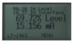
If you have purchased a JMT with the dual float option enabled, it will be done so by default, and cannot be changed without factory assistance. The unit must have two (2) floats to function properly and will flash "LOST SIGNAL" if second float is not installed.
