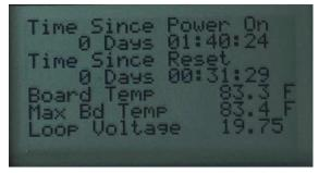
Diagnostics will show information regarding the transmitters operating temperature, loop voltage, and time since last reset or power on.
