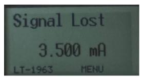
In the event the instrument is no longer detecting a magnetic field from the float (in single level or in dual level), "Signal Lost" will flash between black and white on the display. The output current is set to the NAMUR- 43 standard of either 3.5 mA, or 21 mA, based on user selection.
