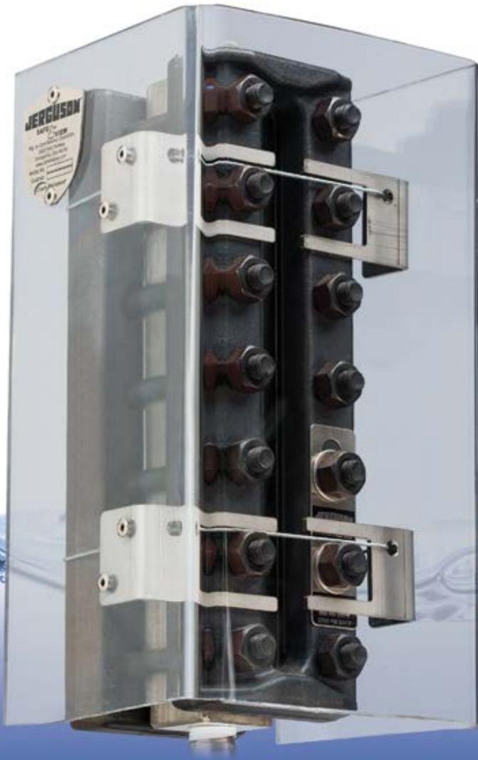
SafeView Shields protect operators from potential flat glass gage high pressure leaks. Although armored glass liquid level gages are extremely reliable, leaks can occur due to deferred maintenance or the rigors of continuous operation under high pressure. Erosion of armored gage glass, for example, is often invisible without inspection of the disassembled gage.
