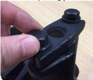
2) Carefully remove the old nipple packing cartridge from the valve body chamber. You can use a small flat screw driver or pointed tool to remove the cartridge. Use caution that the packing chamber does not get damaged.
