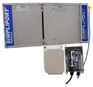
Illuminators for the Simpliport 180 are available for NEC-500, Class I, Division 2 and NEC-505, Class I, Zone 2 applications, for use with the same Viewing Hoods as our ordinary location illuminators. Models are available with local and remote Power Supplies for installer convenience. The maximum distance for the remote power supply to light is 1000' (305M).
