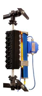
Illuminators for Flat Glass Gages are available for Hazardous Locations, including IECEx and ATEX applications. Individual DuraStars are required for each gage glass window section. The illuminators may not be "daisy-chained" for Hazardous Location applications. However, the installer may use a single power source routed through an appropriate junction box to power the individual illuminator power supplies.
