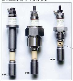
The FBRZ type has been designed for specification or retrofit into any Clark-Reliance instrument designed for 3000 PSI.
