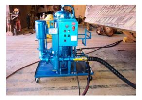
Custom designed Portable Filtration Systems provided by Oil Filtration Systems, Inc. are equipped with high-efficiency 7-Micron filter elements rated Beta©>1000 per ISO 16889, meaning that 99.9% of all particles 7-Micron and larger are removed in a single pass. Since both oils must be reclaimed to meet or exceed OEM recommended cleanliness levels during a normal 4-hour maintenance interval, a relatively high flow rate on the Portable Filtration Systems is required.
